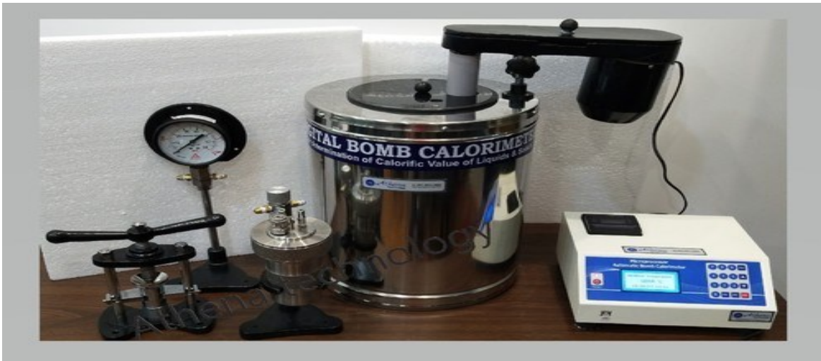
Fig 4 Bomb Calorimeter for calculating gross calorific value (GCV)
