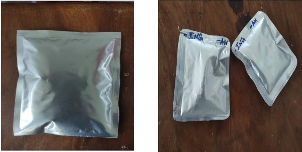
Figure-3. Aluminium based encapsulated pack for cooling device (a) Organic Pcm (b) Inorganic Pcm pouch.
