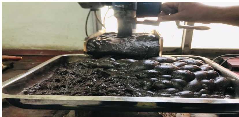
Figure 2. Copper concentrate coming out in upper float of Flotation Cell.
