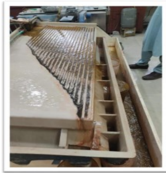
Figure 3. Shaking table used in experiment
