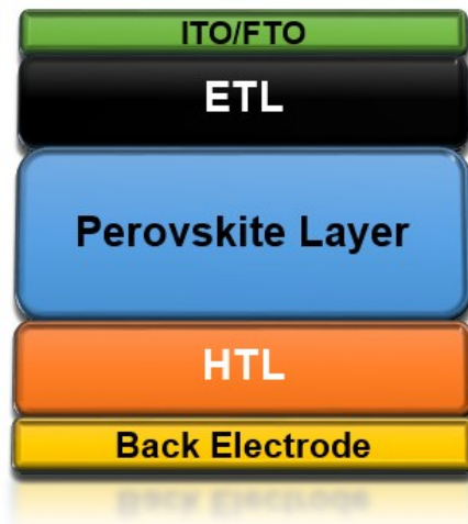
Figure 1: Layer Structure of Perovskite Solar Cell
